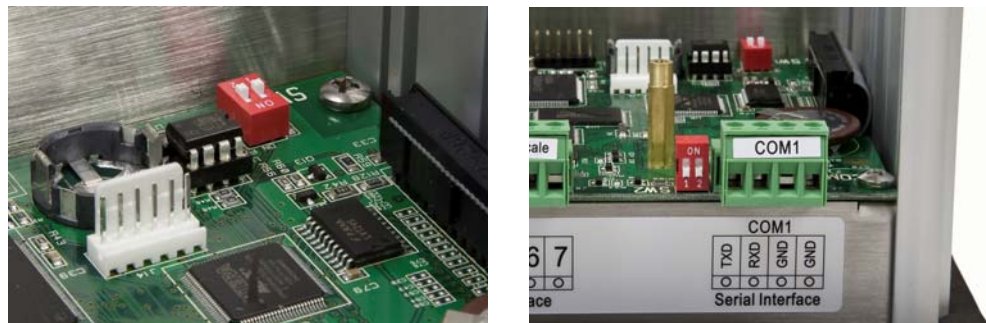
Figure A-35: SW1 (left) and SW2 (right) Locations
