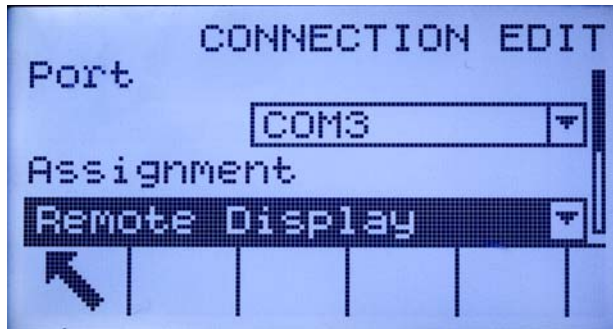
Figure 3-10: COM2/COM3 Connection Configured for Remote Operation
