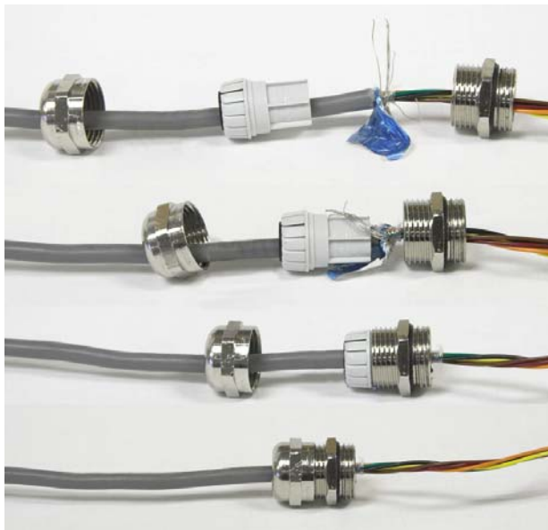
Figure A-16: Shield Termination at Gland
