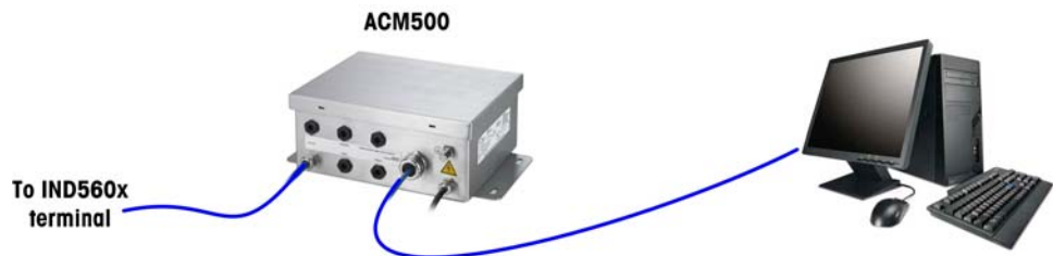
Figure D-1: Connecting the IND560x to a PC with a Crossover Cable
